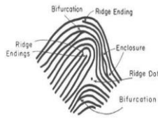
Fig 1.3.2: An example of a ridge ending and a bifurcation Source: H. Chang, D, 1999
